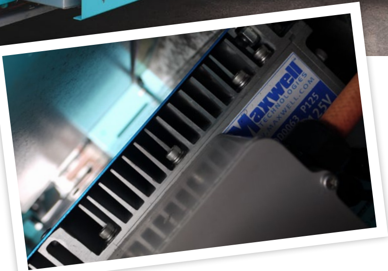
ABOVE & RIGHT: The blue box for energy storage on the side of the vehicle indicates that this is not an ordinary Konecranes reach stacker
