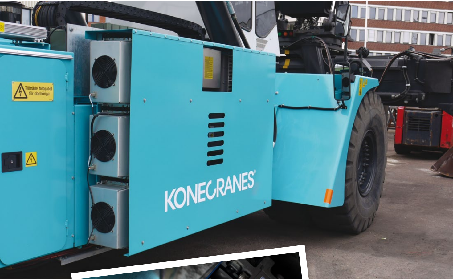
ABOVE & RIGHT: The blue box for energy storage on the side of the vehicle indicates that this is not an ordinary Konecranes reach stacker
