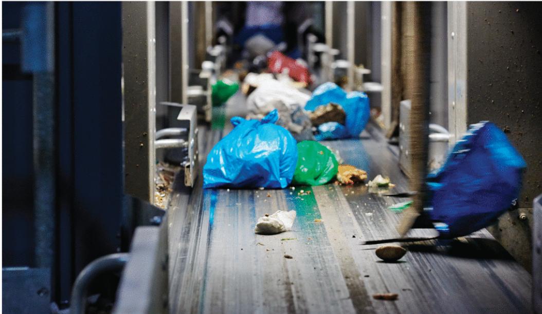
Blue and green bags are identified using industrial vision technology and removed from the stream
